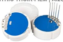
■ Range: 0~2bar~100bar/600bar ■ Size:18mm\*6.35mm; 18mm\*3.5mm ■ Diaphragm Material: Ceramic Al2O3 96% ■ Power Supply: 2-30V ■ Long Term Stability: 0.3%/FS ■ NTC Thermistor ■ Working Temperature: -40...+135 °C
