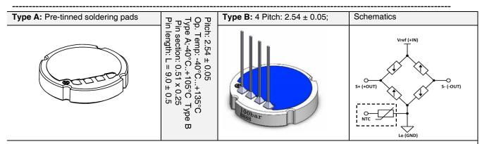
1. Storage Conditions: Store at 10~35°C with ≤70% RH. Avoid places that are too hot, exposed to direct sunlight, dusty, or have corrosive gases. The metal pins can easily oxidize in the air, so it's recommended to use the product within 10 days after unpacking. Under proper storage conditions, the soldering validity is 12 months. If stored for more than 12 months, the ceramic core needs to be rechecked for solderability and can only be used if it passes inspection.
