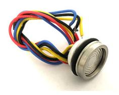
Range: -100KPa-10Kpa~3.5MPa Overload Pressure: 150%~300% Accuracy: 0.1-0.2%%/FS Welded Flat Base
