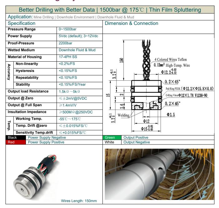
Connect and power on the device in strict accordance with the prescribed wiring method and power supply voltage as outlined in this specification. The maximum measured pressure must not exceed 150% of the rated value, and the burst pressure must not exceed 300% of the rated value. The measured medium should consist of gas or liquid that is non-corrosive to stainless steel.
